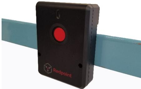
Vehicle Mount Tag mounted on bar
